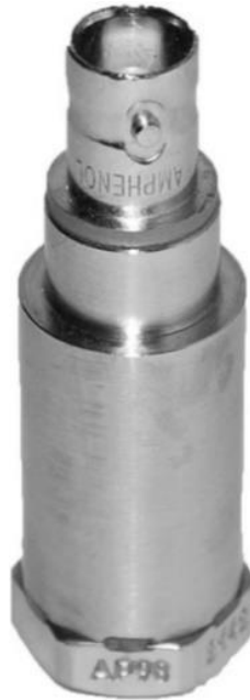
Figure 4. used accelerometer for doing research
