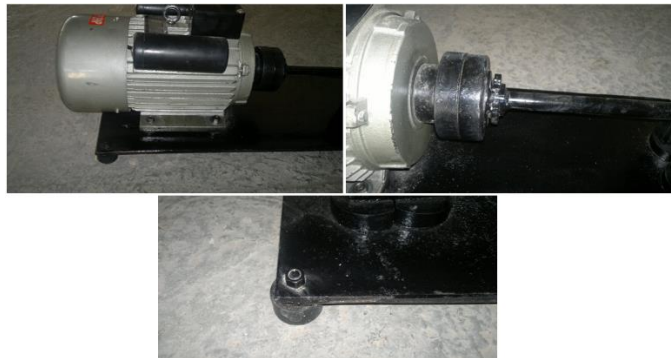
Figure 2. Couplings, electrical motor, bumpers and rubber base used to make the system operational
