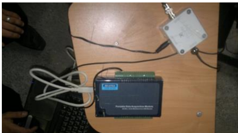
Figure 5. View of the amplifier and ADC used in research
